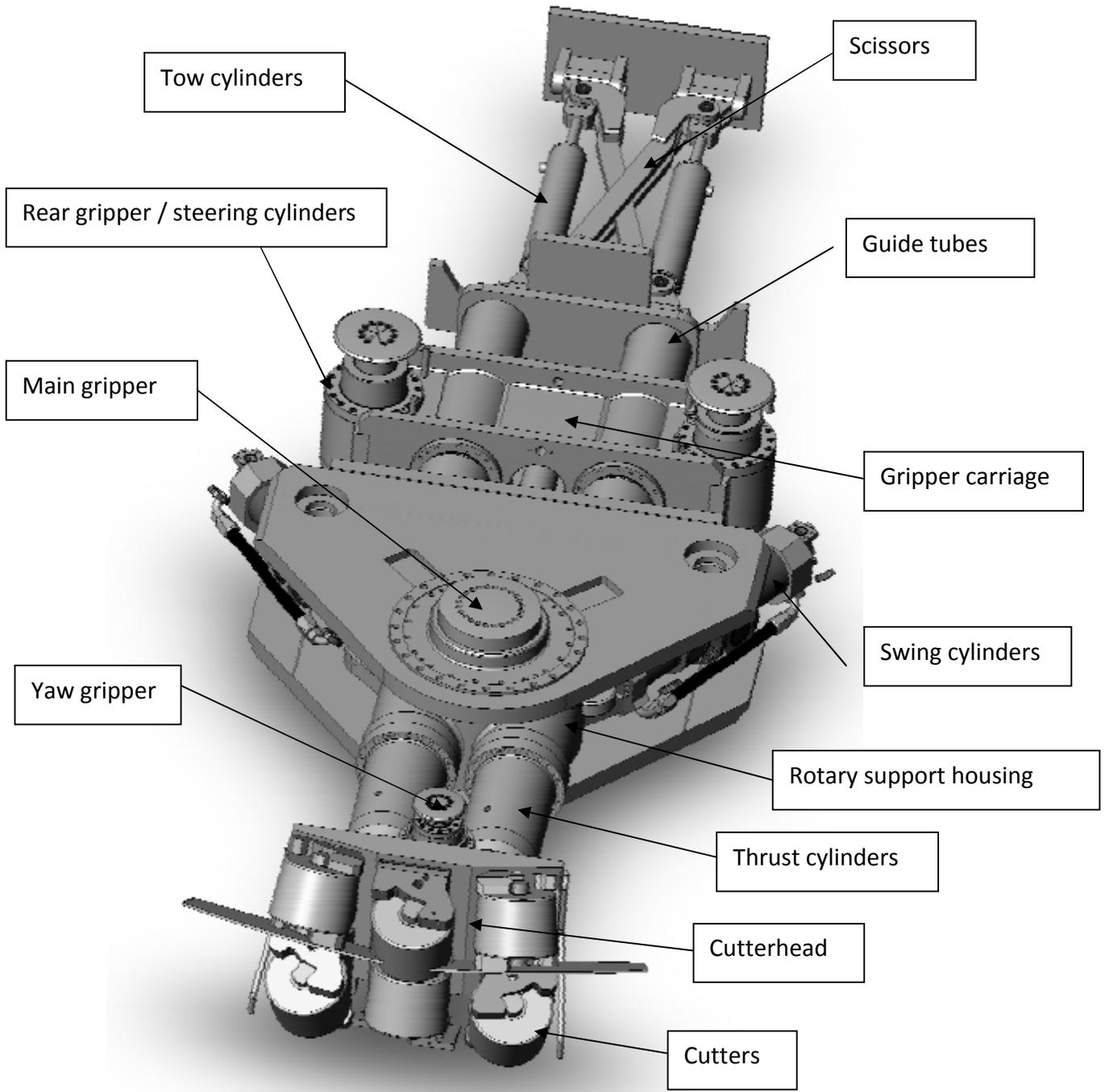
Figure 2.1 : Machine assembly
